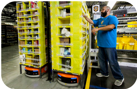
For over a decade, Amazon’s Kiva robots (pictured here bringing a pallet of products to a warehouse order-fulfillment packager) have been central to their competitive edge, with over 500,000 robots now in use.
