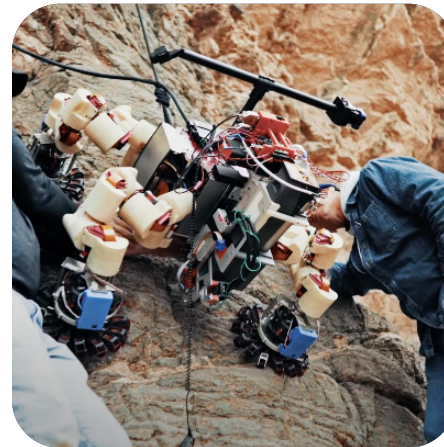
Originally developed by NASA for use in zero gravity, engineers at Amazon are using microspine-gripper technology in conjunction with machine learning to teach their warehouse bots how to handle individual products with a degree of dexterity still largely the domain of human hands.
