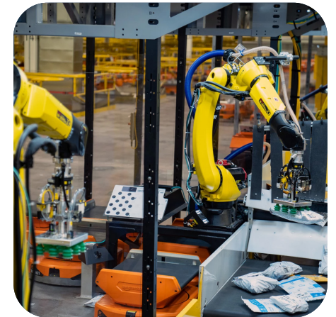
Originally developed by NASA for use in zero gravity, engineers at Amazon are using microspine-gripper technology in conjunction with machine learning to teach their warehouse bots how to handle individual products with a degree of dexterity still largely the domain of human hands.
